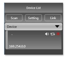
When using TCP control, there is a situation that only one point is displayed after scanning, but you can not connect the device. In this case change the IP address of the device to the same network range as the computer.
