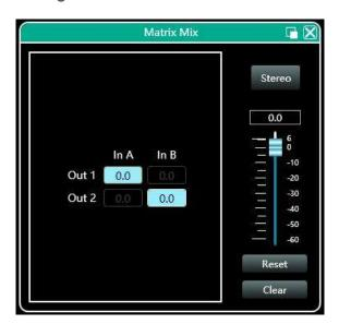
In the above figure, input channel (on top side) corresponds to output channel. The value box with a value is mixing key of channels. When the mixing key is green (double-click the value box to switch the state), the input channel and output channel signal realizes the mixing function.
