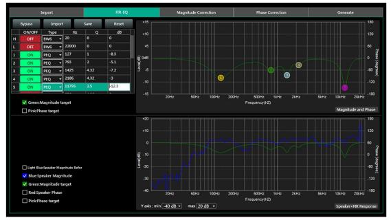
There are High pass filter and low pass filter for setting frequency divider, and 15 bands of PEQ \ LSLV \ HSLV to adjust magnitude. Try to set a linear magnitude of target speaker.
