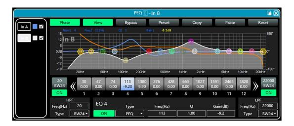
As shown in the figure above, the left side is the interface switching button for each channel. Click to switch the EQ channel, and the color is the currently selected channel. is the curve color of the EQ channel. For each channel's EQ curve display switch, check it to enable it to display the curves of other channels in the current channel interface.
