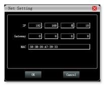
Set the IP address of the device. Refer to the IP showed in the bottom of the software. (the first 3 digits xxx.xxx.xxx. should be the same as the computer.
