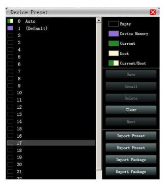
**Save**: select the saved gear, save all the parameter of the current automatic gear of the machine to the device preset (2~30 Preset bit).
