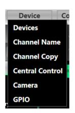
**Devices**: view or modify the software version information, device name and device IP address of the upper and lower computer of the device. **Channel name**: set the name of each input and output channel. **Channel copy**: copy device input and output channel parameter, can realize cross-device copy parameter (Note: the same type of device is re-
