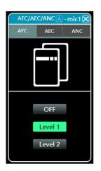
Matrix processor provides AFC (acoustic feedback control) function for microphone. With two level to select, user can control howl round easily when setting each microphone;
