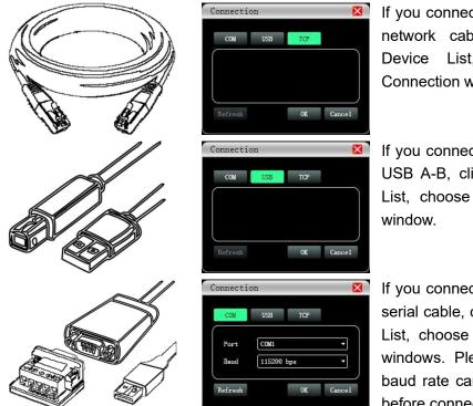
If you connect the device by using network cable, click Setting in Device List, choose **TCP** in Connection window.
