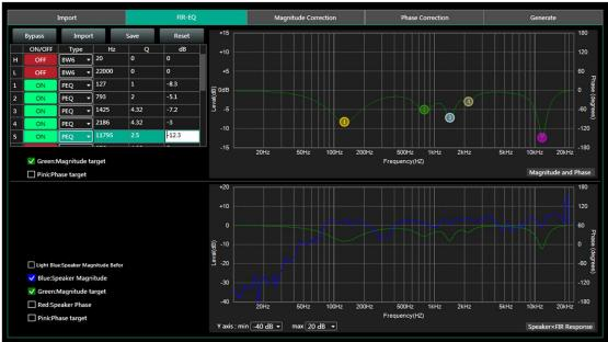
There are High pass filter and low pass filter for setting frequency divider, and 15 bands of PEQ \ LSLV \ HSLV to adjust magnitude. Try to set a linear magnitude of target speaker. Mark: changing FIR magnitude doesn't effect its phase.
