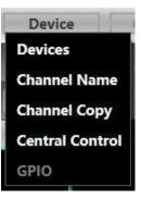
**Devices**: view or modify the software version information, device name and device IP address of the upper and lower computer of the device. Set password of device.
