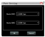
**Port**: set the connection mode, port number and baud rate, confirm the connection mode and then select the corresponding port.
