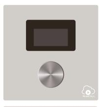
**MDM-CON1** is aPoE powered controller which communicates using UDP protocol. Fully configurable in the software, equipped with 1.31" OLED display. It offers various audio control capabilities such as volume adjustment, mixing, room combining and scene switching.
