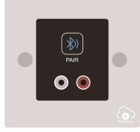
**MDM-BT** is a wall panel that supports mutual conversion between Bluetooth signals or stereo signals and Dante/AES67 network digital signals, and the Bluetooth signal has priority. Connect with mobile phones, iPads and other devices through Bluetooth, the received audio is converted into the Dante<sup>®</sup> network. The papel is powered by PoF, and a network cable is used for power supply and
